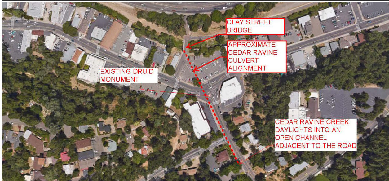
CEDAR RAVINE CULVERT ALIGNMENT
